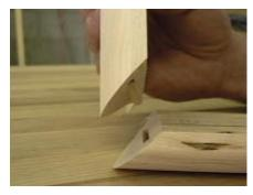
Figure D - Mitered corners joined together with biscuits
